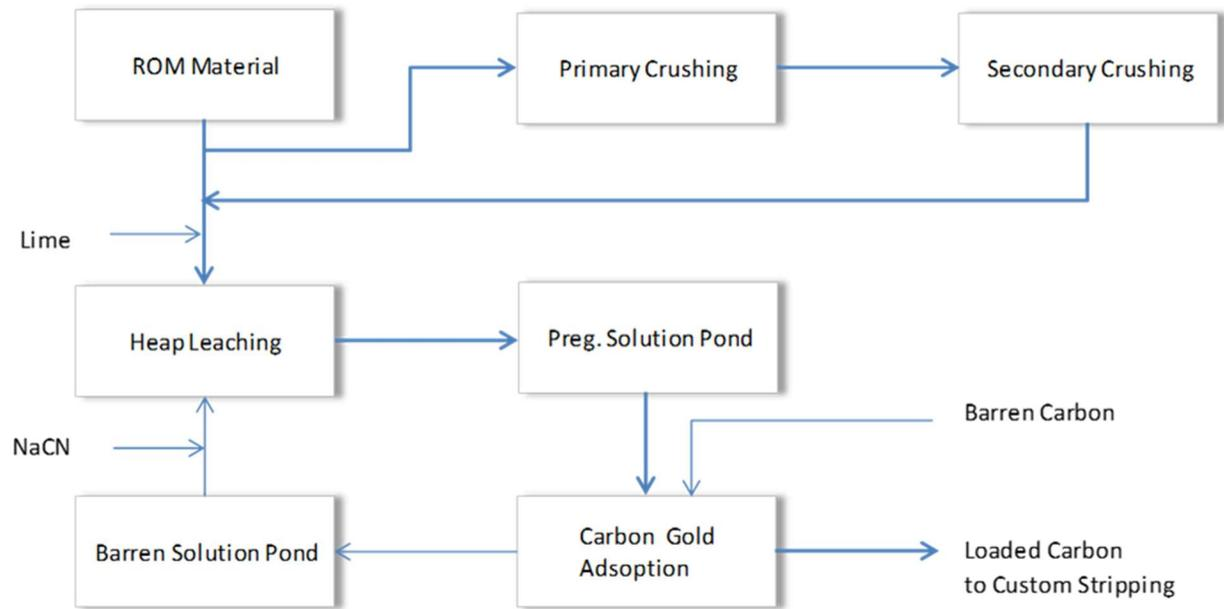
**Figure 17-2: Process Plant Layout (Load Carbon)**
