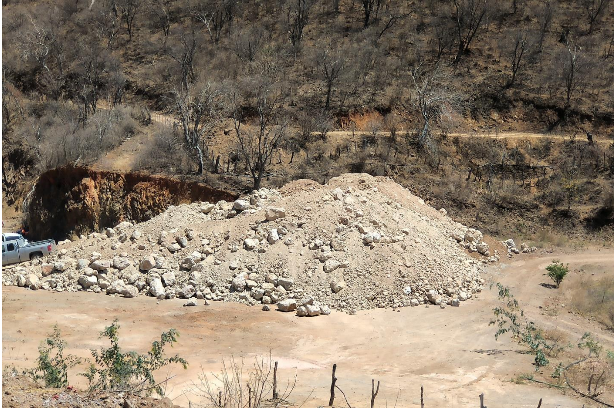
Photo 2 – Stockpiling of mineralized material in preparation for screening and crushing
