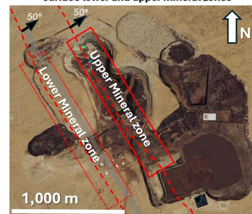
Plan View, pit, infrastructure, and projected to surface lower and upper mineral zones
